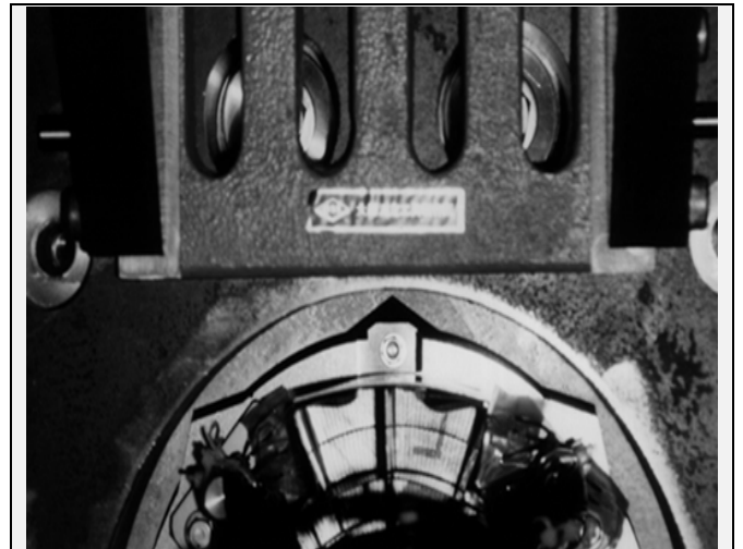
Fig. 3. The short model in the yoking press prior to final assembly with the gap between collar and yoke visible.
