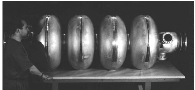
Fig. 1: 4-cell Copper substrate cavity (before sputtering). 256 of those are at present installed in LEP.
