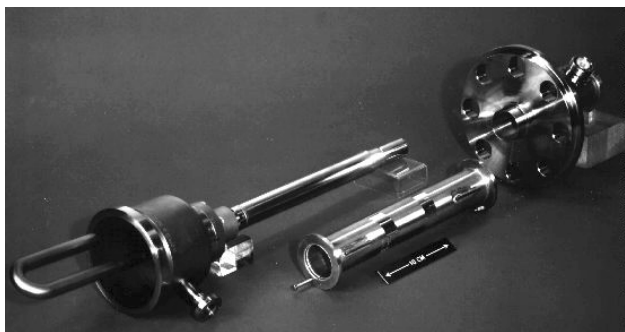
Fig. 4: Hook-type HOM coupler made of Nb (left) and parts of the rigid coaxial output line
