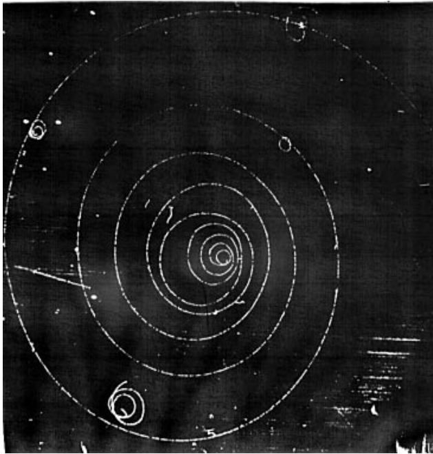
Fig. 4.8.: Muon track in magnetic field in matter.
