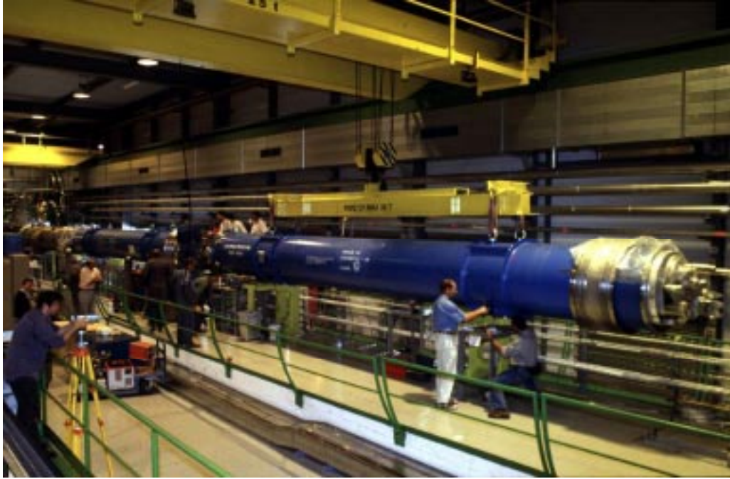
Figure 24: Test string of prototype magnets and quadrupole.
