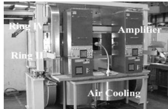
Figure 3: C02 test mount for PSB rings II and IV
