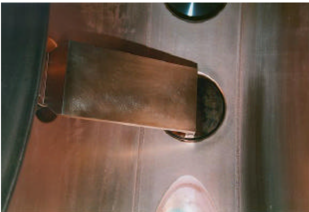
Figure 3: Power coupling loop mounted inside the cavity.
