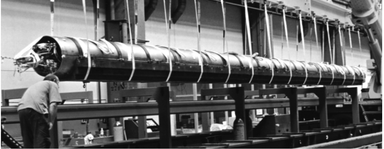
Fig.4. The prototype ready to be displaced onto the welding bench. The cold mass was assembled and aligned straight. Curvature during welding is imparted by shims placed on the welding bench. The metallic belts are still in place (courtesy of Ansaldo).
