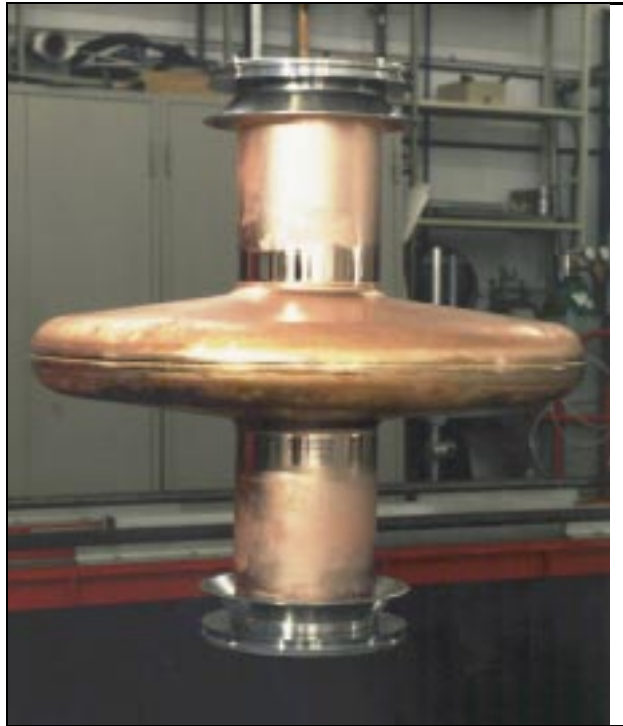
Photo: Copper cavity \beta=0.48 ready for sputtering
