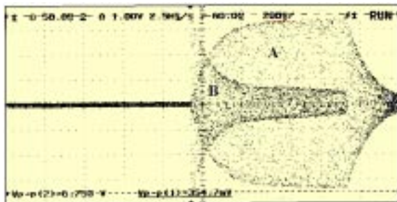
Pulsed RF power A - Cavity field B - Reflected RF power Time scale 200 \mu\text{s} / div
