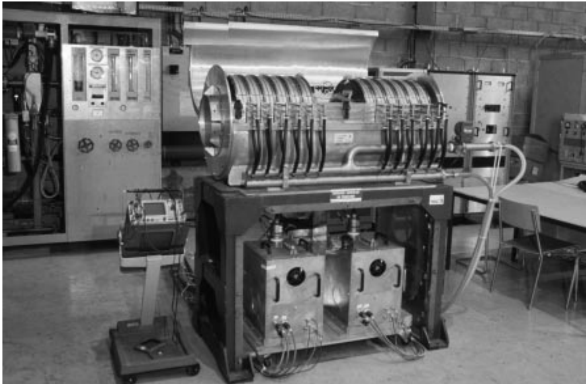
Figure 6: Laboratory set-up at CERN with the tubes TH541 (2x10 kW power installed). At present the configuration has changed, and the new set-up is with the COSY-KFA amplifier and the tubes TH120 (2x50 kW power installed).
