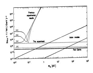
Figure 4. Exclusion plots on the  $g_{a\gamma\gamma}$  vs. axionmass plane. The curve to the left are from Ref. [10]. The letters indicate the following helium gas pressures in the conversion region of a strong magnetic field: (a) vacuum, (b) 55 Torr, and (c) 100 Torr.
