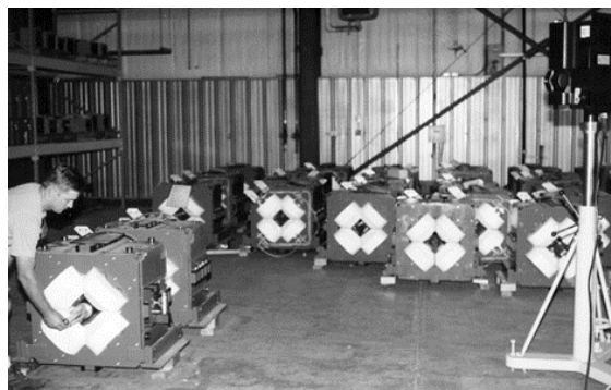
Fig. 54 Fiducialization with laser tracker
