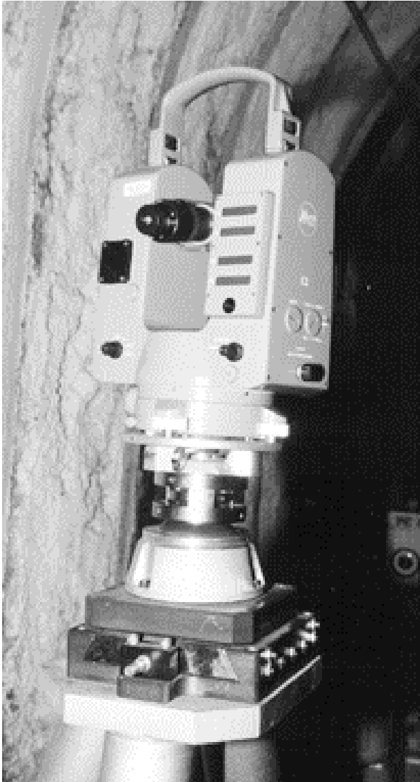
Fig. 19 CERN socket with E2 mounted in sloped tunnel
