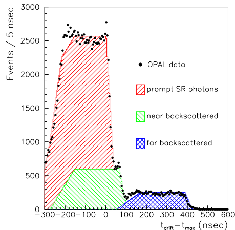
Figure 12: Distribution of arrival times (relative to the maximum drift time for the hit wire) of synchrotron photons in the OPAL vertex drift chamber. The data points are data from the 1992 run. The different cross-hatched areas represent the contributions from prompt and near- and far-backscattered photons. The time delay for near-backscattered photons was 60 ns, corresponding to backscattering from a distance of about 9 m. For the far-backscattered photons, the time delay was 385 ns, corresponding to about 60 m.
