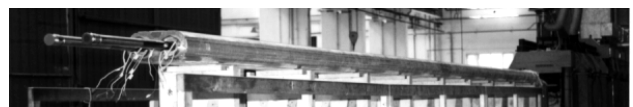
Figure 2: Collared coils of the first 15 m long magnet (courtesy of Ansaldo Energia S.p.a.)
