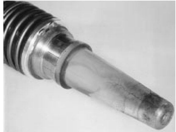
Fig. 6 Connector with traces of corona
