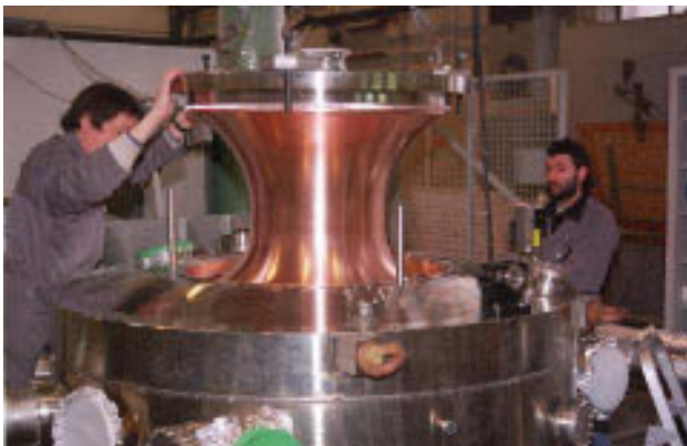
Figure 1: Mounting the center electrode into the cavity.
