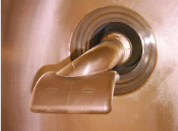
Figure 4: The capacitive power coupler mounted inside the cavity. The form is adapted to the electrode, which is not mounted.
