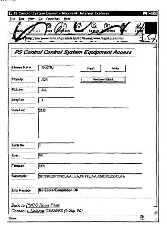
To use the page one should fill in the parameters Element Name, Property, PLSLine, and click for instance the 'Hotlink' button. The *DataField*, *CycleNo* and *User* labels will be refreshed in synchronism with the PS timing system (PLS).
