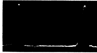
Fig. 4 : typical bunch signal response : BW : 110 MHz 100 mV, 20 ns/div.
