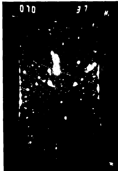
Fig. 27. H_2 + \frac{1}{2}\% \text{ CH}_4 before coating of the central high voltage cathode mesh (660 torr); 25 \Omega chamber.
