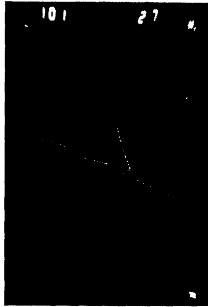
Fig. 17. Typical cosmic ray in the streamer chamber (track length \sim 35 cm). He at 760 torr.
