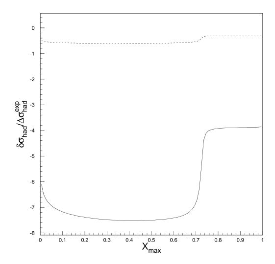
Figure 1: Sensitivity of the hadronic cross-section to  $f_{DW}$  (full line) and  $f_{DB}$  (dashed line), as a function of the fraction  $x_{max}$  of center-of-mass energy carried away by initial state photons.
