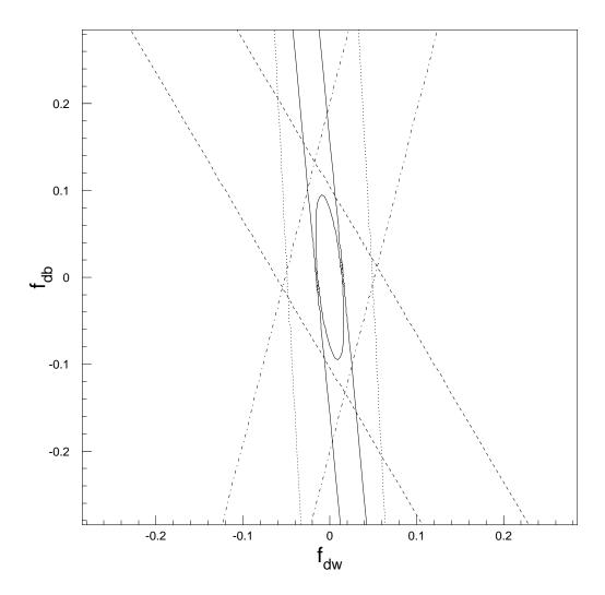
Figure 3: Constraints in the  $f_{DW}$ ,  $f_{DB}$  plane resulting from the measurements at NLC (1 experiments, 20 fb<sup>-1</sup>) of  $\sigma_{hadrons}$  (full lines)  $\sigma_{b\bar{b}}$  (dotted lines),  $\sigma_{\mu}$  (dashed lines), and  $A_{FB}^{\mu}$  (dash-dotted lines). The ellipse represents the one standard deviation (39% C.L.) constraint resulting from the combination of the four above measurements.
