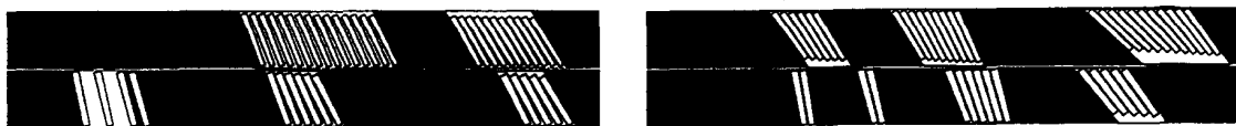
a) spaces to be filled to restore the outer cylinder of each coil layer b) spaces to be filled to restore the inner cylinder of each coil layer
