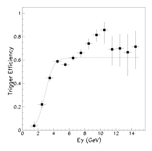
Figure 1: Single photon trigger efficiency in the HPC as determined from Compton scatter events. The curve shows the result of a fit to the function  $\epsilon(E_{\gamma}) = A/(Be^{-E_{\gamma}*C}+1)$ , with A = 0.64 ± 0.01, B = 68. ± 30., and C = 1.41 ± 0.15 GeV<sup>-1</sup>.
