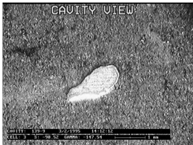
Fig.2: Inner cavity surface with 1.5 mm long irregularity.
