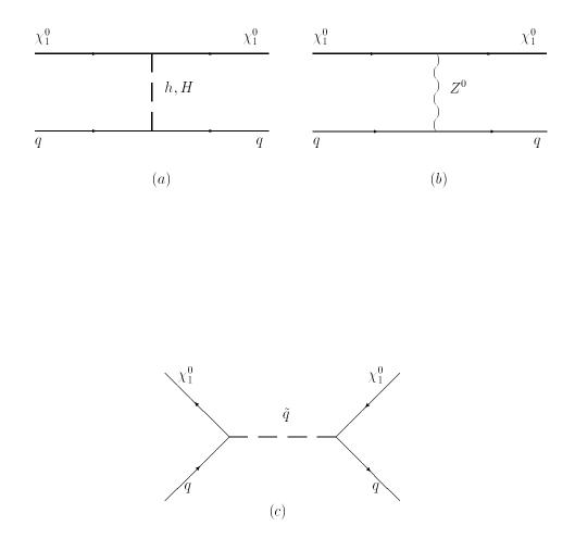
Figure 1: The Feynman diagrams for the elastic  $\chi_1^0$ -quark scattering process, which occurs via *t*-channel *h*, *H*- and *Z*-boson exchange (a, b) and via *s*-channel  $\tilde{q}$ -exchange (c).
