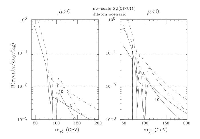
Figure 3: The calculated scattering rates for the Ge (solid lines) and Pb (dashed lines) dark matter detectors in no-scale  $SU(5) \times U(1)$  supergravity – dilaton scenario for tan  $\beta = 2, 10$ . The horizontal dotted lines represent the detector sensitivities of 0.1 and 0.01 events/kg/day. The dips in the rates correspond to a suppressed neutralino relic density when the Z and h poles in the neutralino pair annihilation are encountered.
