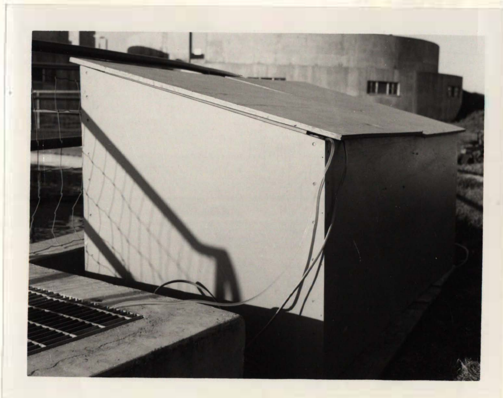
Figure 10. Insulated enclosure for pilot plant equipment.
