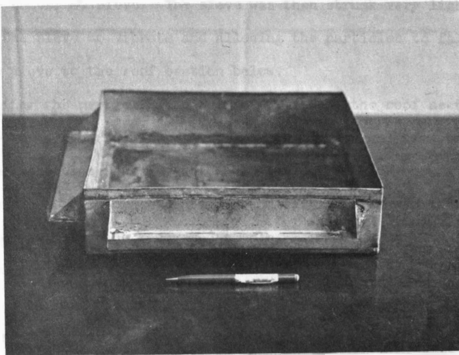
Figure 4 A Typical Sieve for Distributing the Particles
