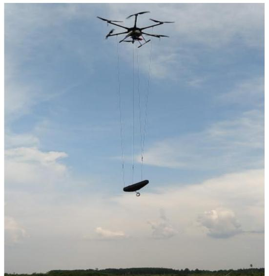
Figure 2: Circada drone flying the UMT MFAM Magpike over a test-site in Ukraine
