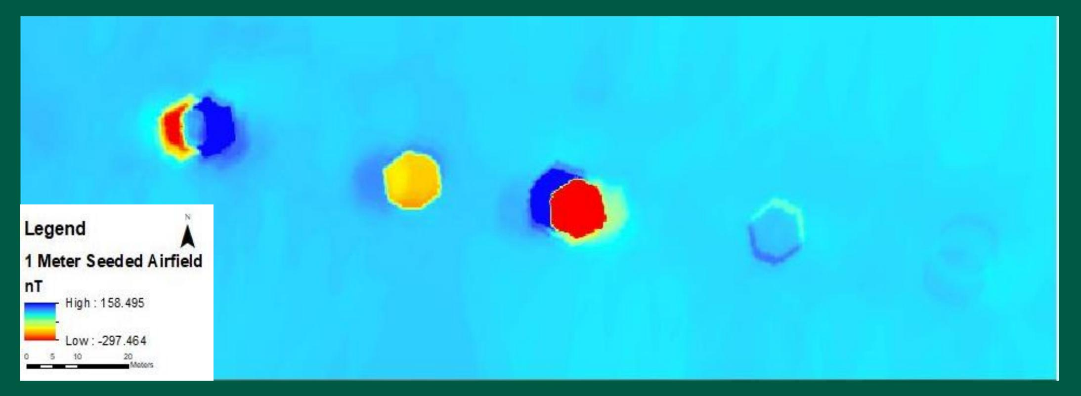
Figure 4: 1-meter magnetometer data collected over an airfield in Chernihiv, Ukraine. The trial was completed at ground level with a handheld magnetometer. Being closest to the surface resulted in the clearest imaging, indicating that there are six anomalies in the survey area.
