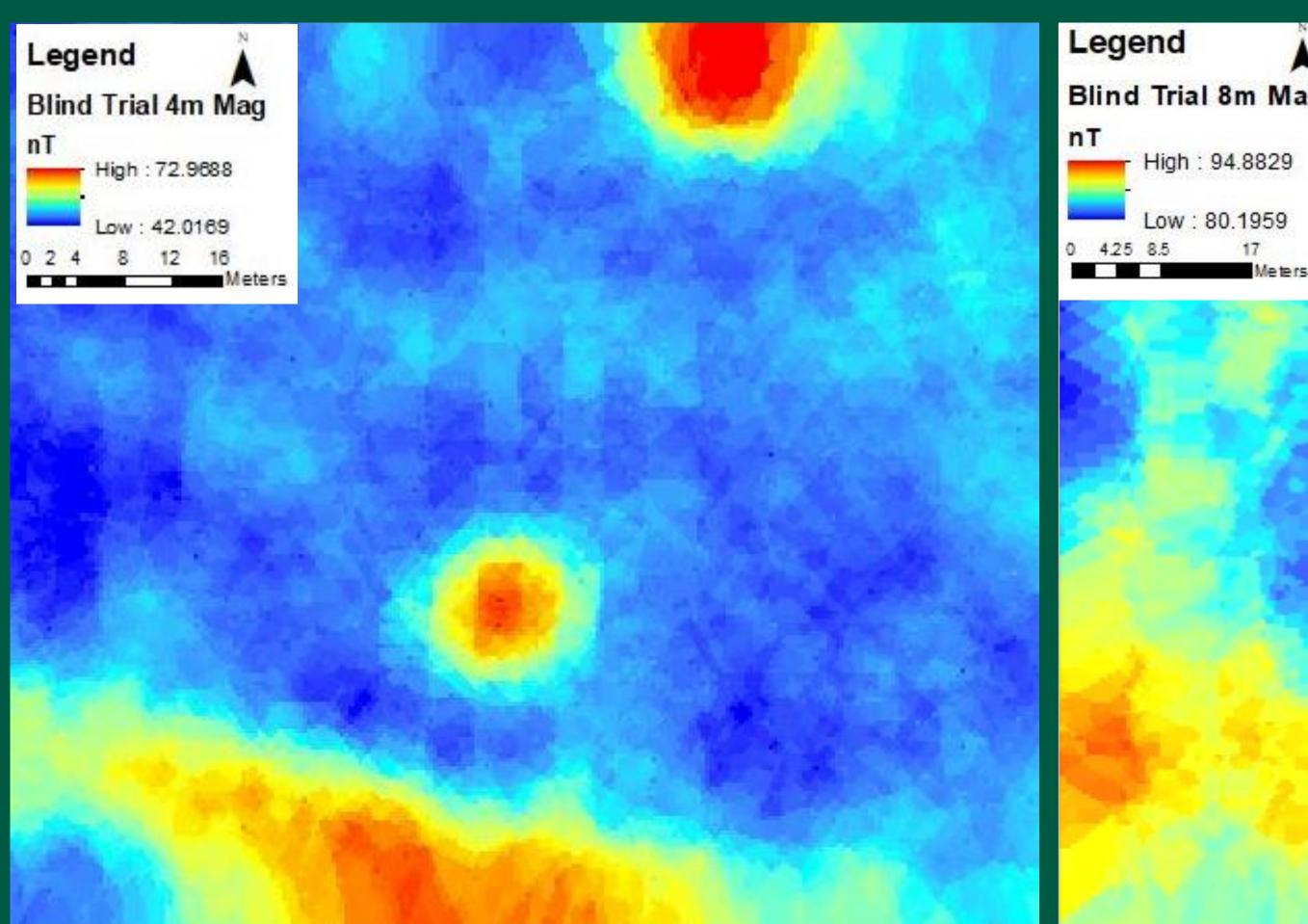
Figure 3: Aerial images of unexploded 122mm 9M22U rockets collected from Ukraine. In the left image, the magnetometer is collecting data from 4 meters above ground level, while the right image depicts data collected at 8 meters above ground level. The two buried rockets are identifiable by the circular red spots, with the elongated red spot on the bottom of the image being a road.
