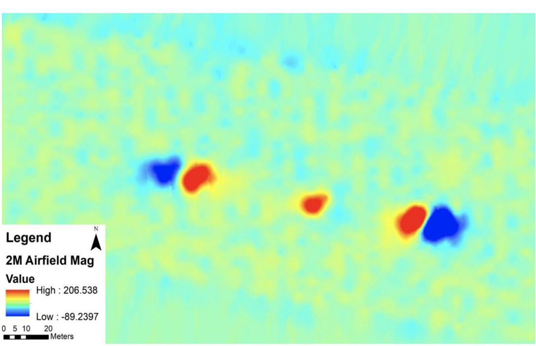
Figure 5: Aerial magnetometer data taken over an airfield in Chernihiv, Ukraine. The magnetometer was oriented 2-meters above the ground. The airfield contained three large unexploded rockets, which are identifiable compared to the background magnetic signature of the site.
