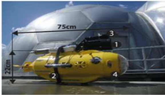
Figure 1. The underwater drone with the attached equipment.
