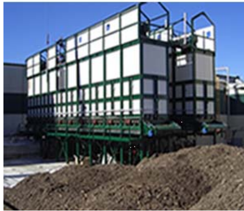
Figure 5.2: Full-scale continuous biodrying reactor
