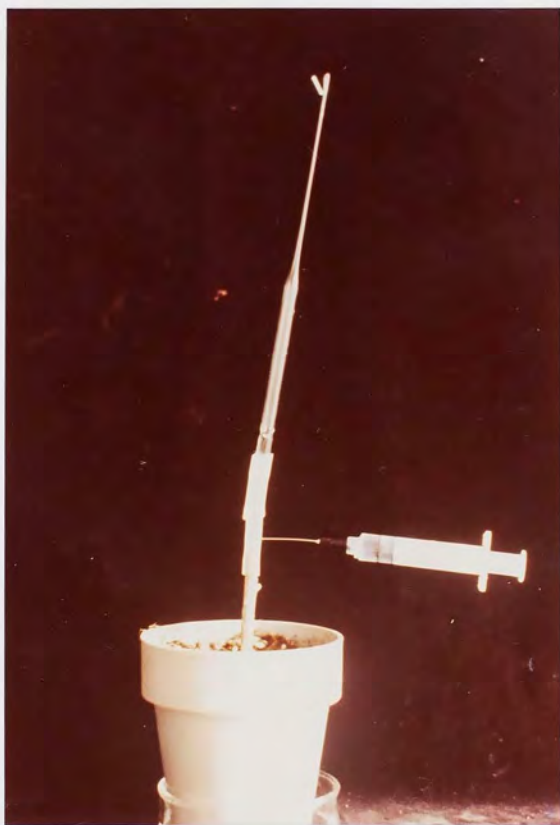
Fig. 2. Method for collecting and extracting xylem fluid exudate from decapitated tomato plants.
