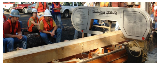
Fig. 1. The Wood-Mizer LT20 TR sawmill being operated by a student, as other students look on to ensure safety protocols are being correctly followed.
