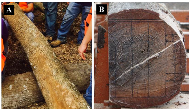
Fig. 2. (A) A hardwood log with evident curvature, which makes estimating the volume of the log and the volume of boards that will be sawn difficult. (B) The cutting solution drawn onto the smaller end of a log. As is evident to the left side, this group had difficulty cutting their boards as initially planned, as they had not accounted for kerf (the wood that will be lost as sawdust due to the width of the sawmill blade) correctly.
