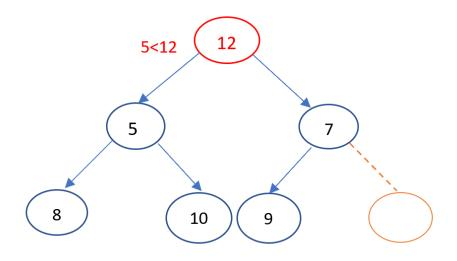
Fig. 15: Example of Min-Heap data structure
