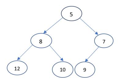
Fig. 17: Example of Min-Heap data structure
