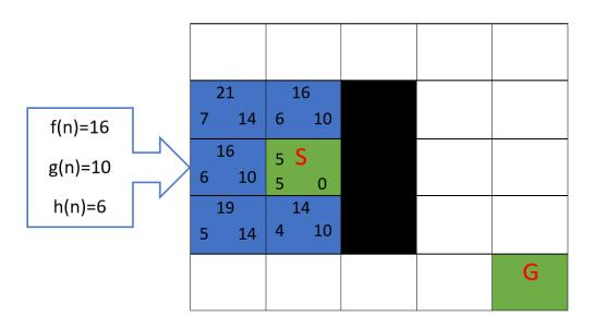
Fig. 9: An example for pathfinding using A\* algorithm
