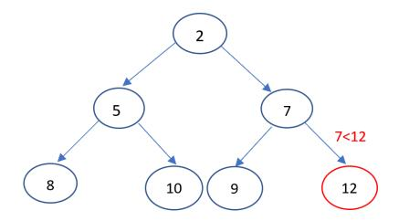
Fig. 13: Example of Min-Heap data structure
