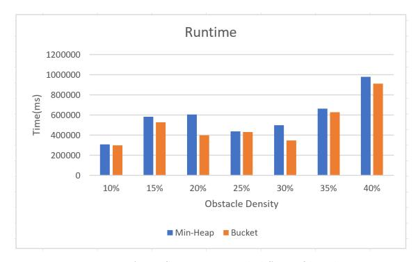
Fig. 30: Runtime of Map Size: 512x512 with different Obstacle Density
