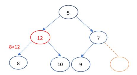
Fig. 16: Example of Min-Heap data structure
