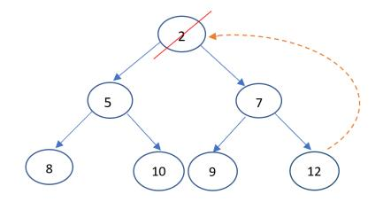
Fig. 14: Example of Min-Heap data structure
