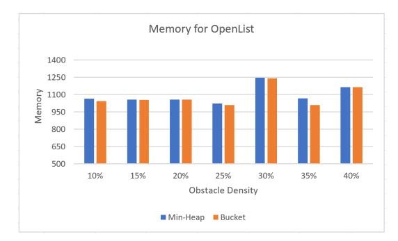
Fig. 37: Memory required for Map Size: 512x512 with different Obstacle Density
