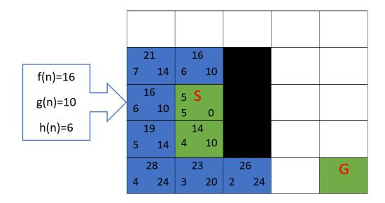
Fig. 10: An example for pathfinding using A<sup>\*</sup> algorithm
