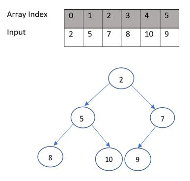
Fig. 12: Example of Min-Heap data structure
