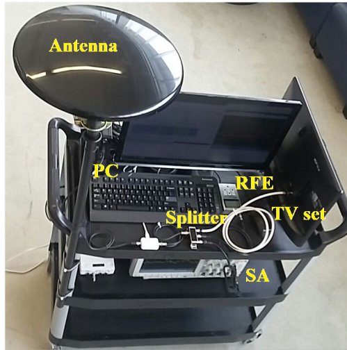
FIGURE 5.2: Portable SSS to sense the spectrum in indoor environments.
