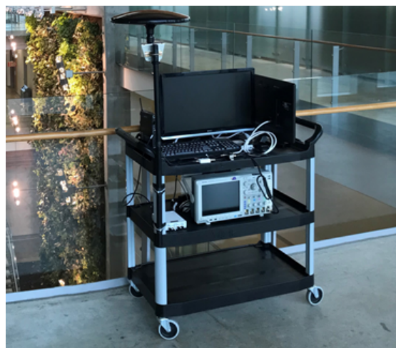
FIGURE 3.5: A portable version of the SSS used to sense indoor spectrum.
