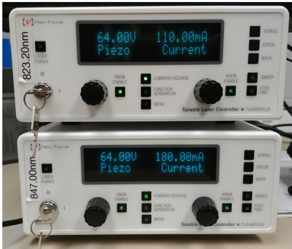
Figure A.1. Front panels of the model TLB-6800-LN tunable laser controllers displaying recommended current supply to the model TLB-6817 Vortex ECDL.
