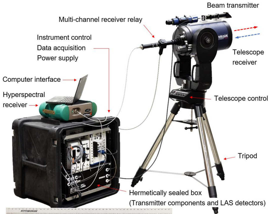
Figure 3.6. Annotated photograph of the Soil Observation Laser Absorption Spectrometer (SOLAS) instrument with major assemblies (transmitter, receiver, data acquisition and control).
