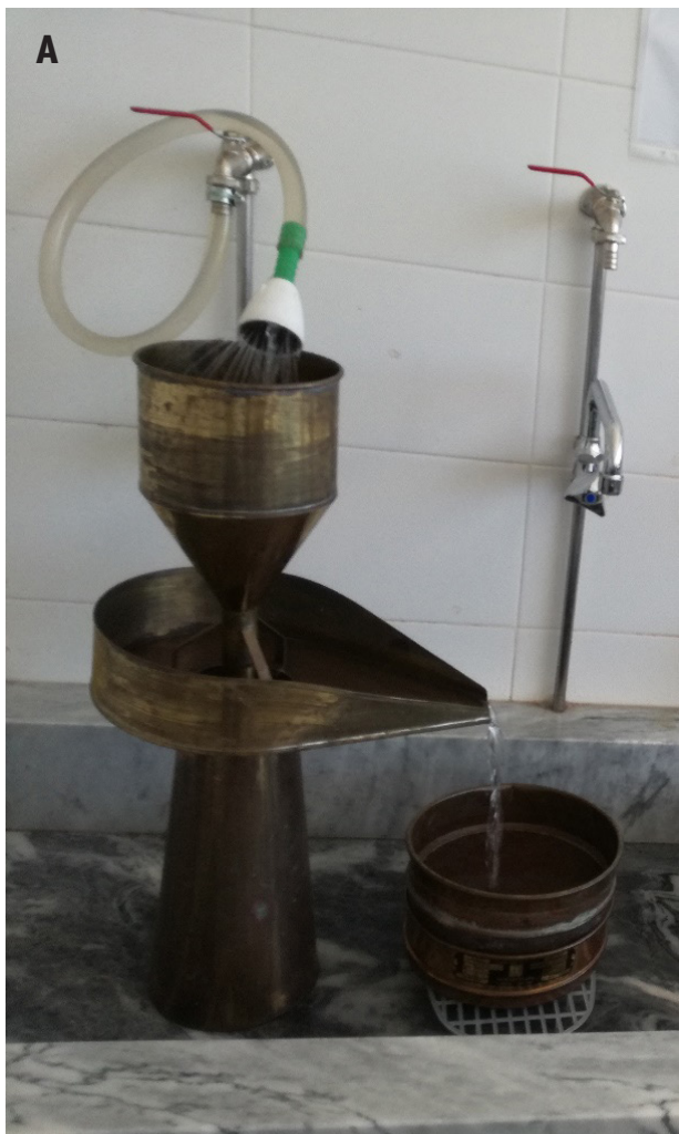
Figure 1 - Extraction methods. A: Fenwick can; B: Cobb's decanting and sieving technique; C: cysts collected.
