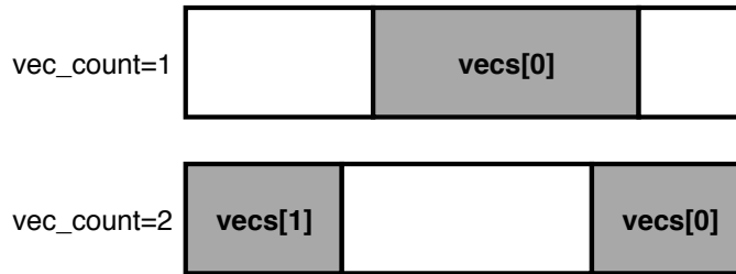
Figure 3.3: Segment representation using iovec .
