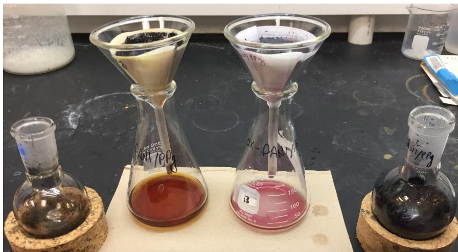
Figure 7.2: Comparison of Qualitative Observations during PANI (left) and ox-PANI (right) Synthesis
