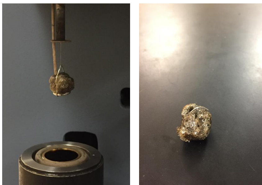
Figure C.6: Expansion of Terpolymer #1 Sample during TGA
