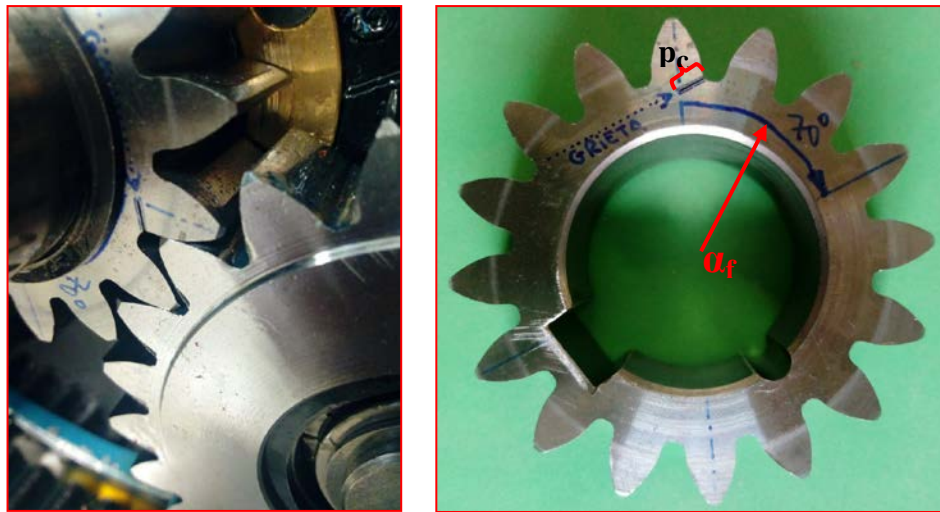
Figure 6. 8. Crack defect located on the test sun
