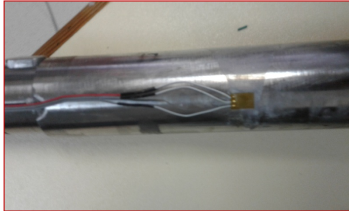
Figure 2. 7. Strain gauge location
