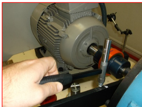
Figure 3. 1. Impact hammer location
