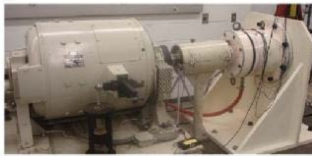
Figure 1. 28. View of the "back to back" train test bench (Ligata., 2007)
