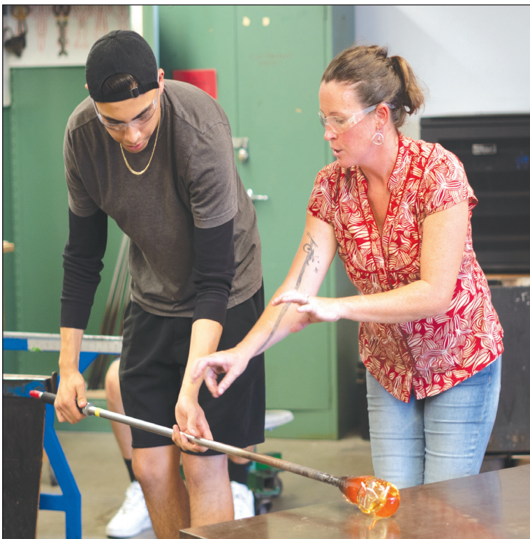
English junior Angel Anaya is guided by Straubing as he rolls molten glass across a steel platform to give it a bulb shape.
