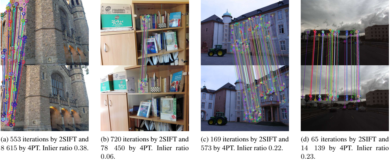
Figure 2: Inliers of the estimated homographies (by 2SIFT) drawn to example image pairs. The numbers of iterations of GC-RANSAC [7] using the 4PT and proposed 2SIFT solvers; and the ground truth inlier ratios are reported in the captions.
