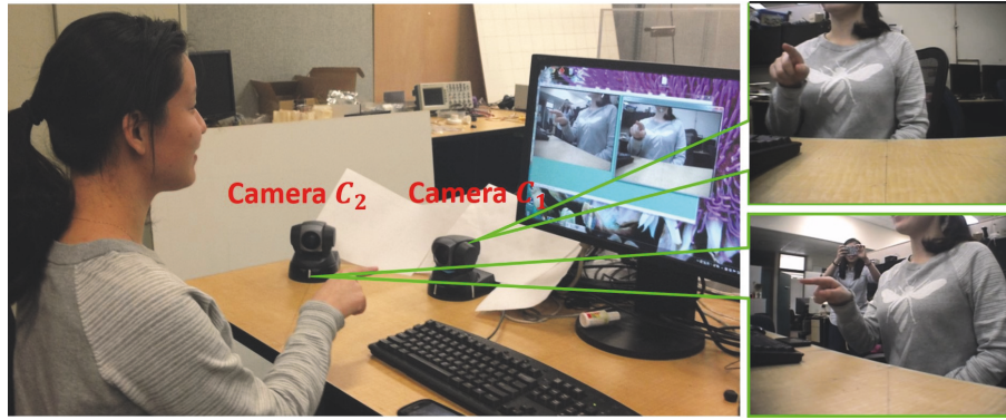
FIGURE 8: The system setup of two cameras. The example frames taken by camera C_1 and C_2 are listed on the left of this image.
