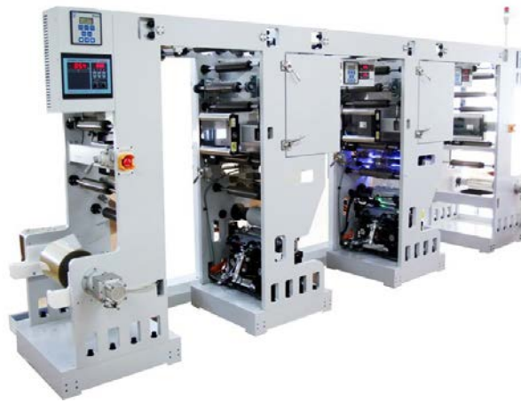
Figure 1 – Actual image of the R2R gravure machine with two printing units
