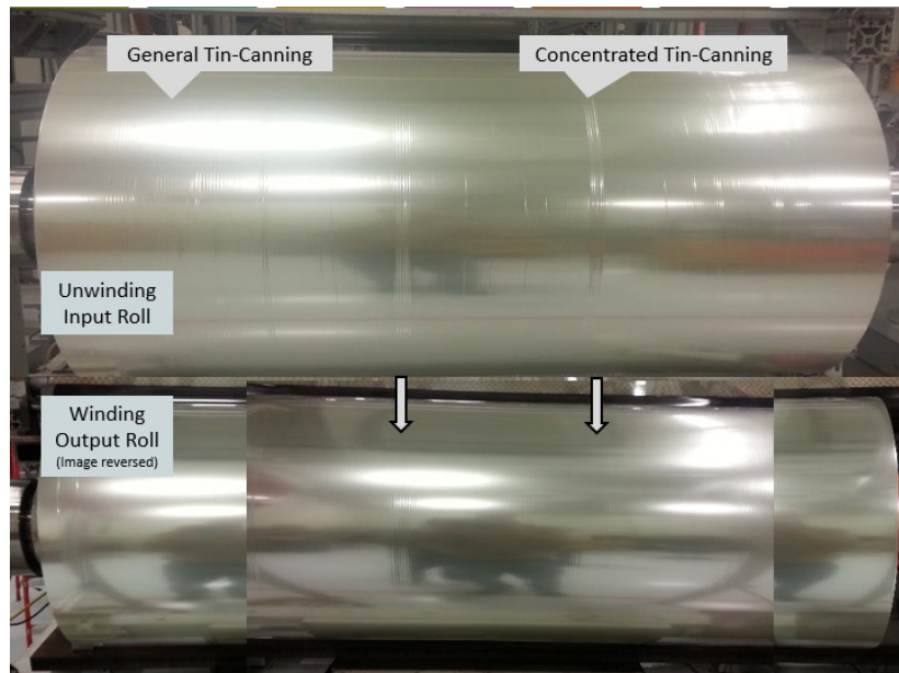
Figure 8 – Tin-Canning Defect Position of Input and Rewound Rolls
