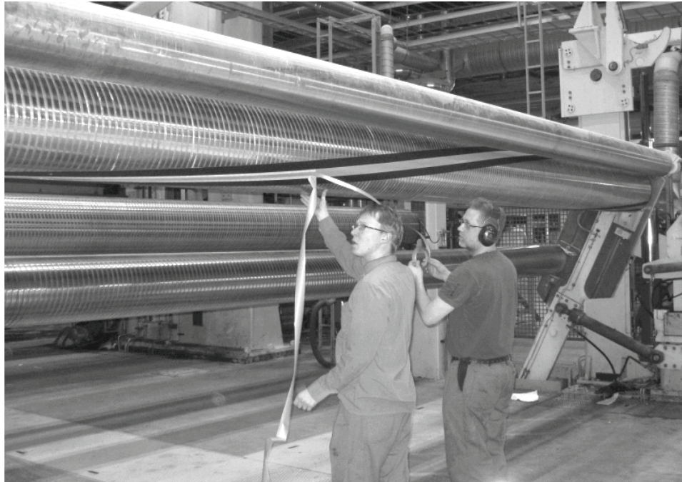
Figure 6 – Installing portable measurement sensors on a roll surface.
