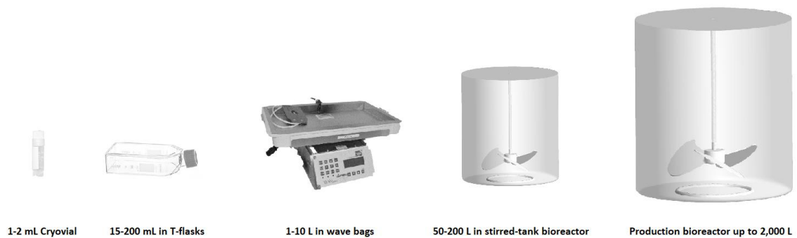
Figure 1.1. Seed-train process of a cell culture production run starting from a few milliliters of frozen cell culture up to thousands of liters.
