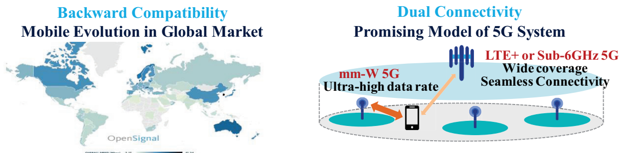
Figure 3. Key principles of 5G system; Backward compatibility and dual connectivity
