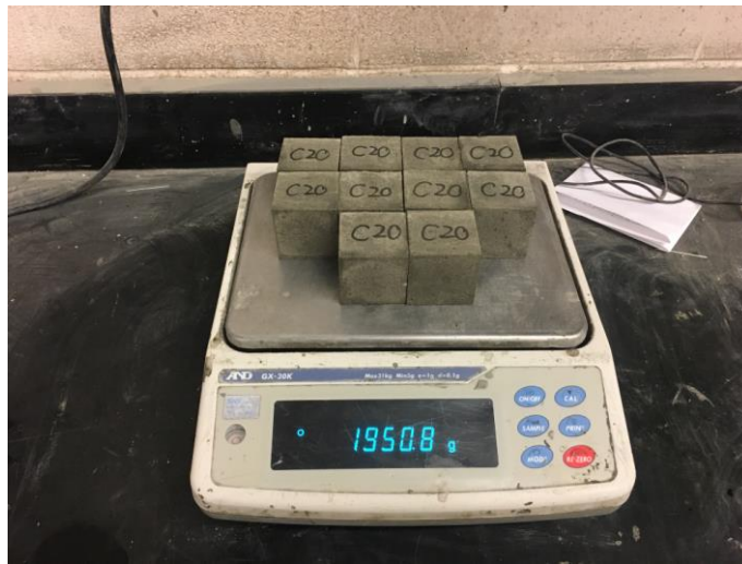
Figure 3.7 Density measurement by the electronic scale.
