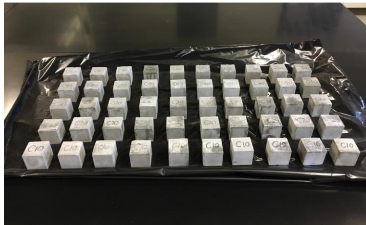
Figure 3.5 Cubic cellular concrete specimens (ASTM C192).
