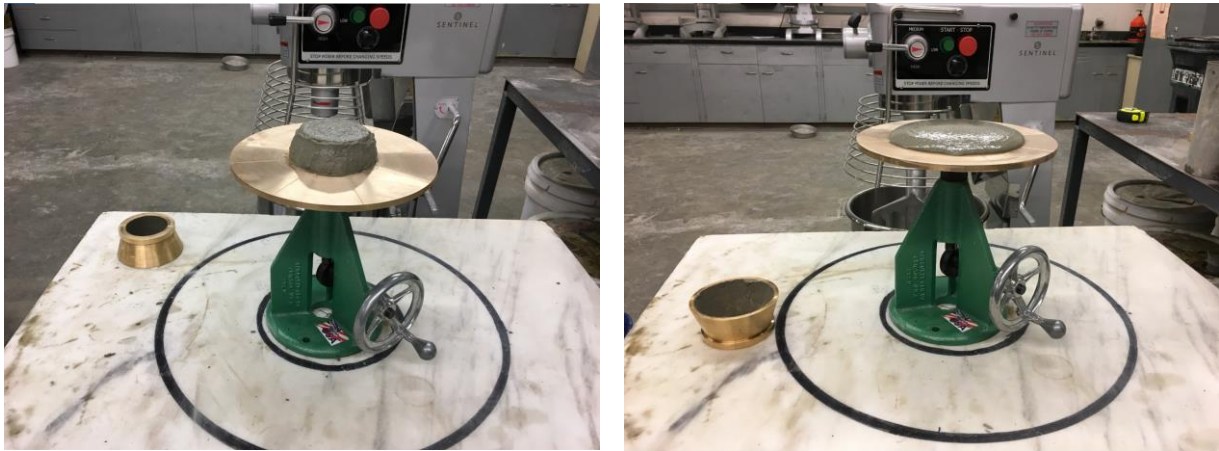
Figure 3.6 Flow table test and accessories to run the test (ASTM C1437).
