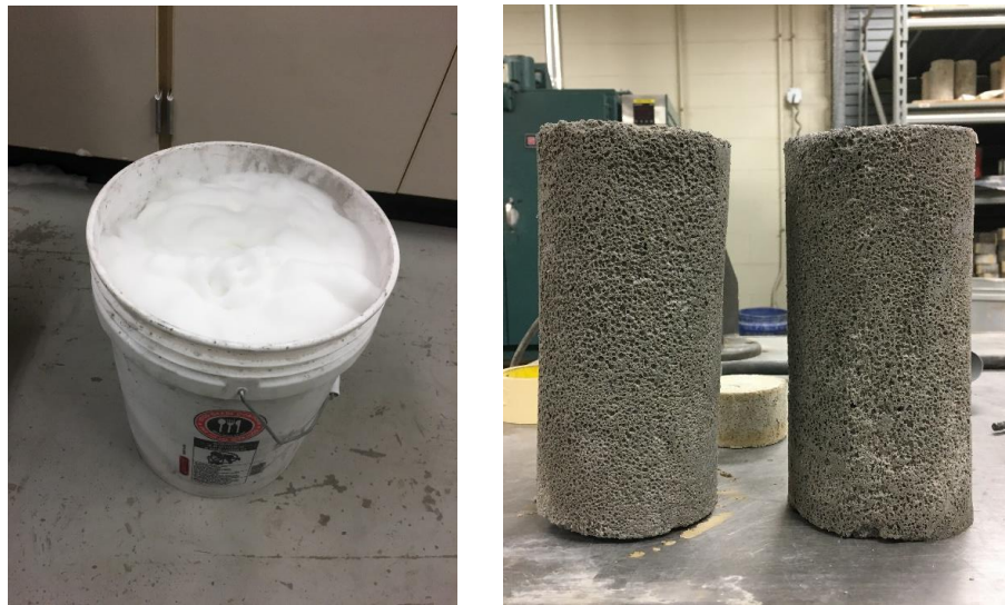
Figure 3.3 The generated foam (left) and cellular concrete specimens (right).
