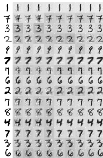
Fig. 1. A sample of digits from the MNIST data set is shown for the original data followed by reconstructions with 40, 60, 80, 100, 120, 140, 160, 180, and 200 hidden layers. The cRBM was trained on the standard training set and the reconstructions are from the testing set.
