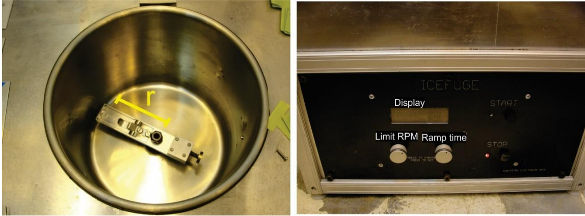
Figure A 2: ( left ) bucket of the centrifuge used to measure ice adhesion. The radius r of the arm is that used with Equation 1 from the main text to calculate adhesion. r is measured from the centre of the centrifuge arm to the position of the ice on the coupon. ( right ) digital display on the icefuge that gives the maximum speed of rotation reached before detachment. The limit RPM dial and Ramp time dial are used to adjust the speed the centrifuge will reach. The same limit and ramp time were used for all samples: 4900 RPM, and 60 sec.
