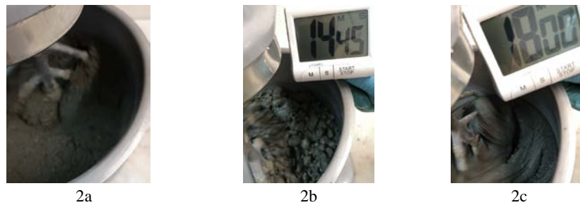
Fig. 2. 1.5 liters mixer used for the mixing process of the UHPC reference mixture.
